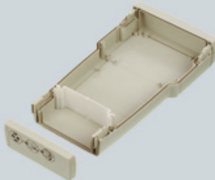
BOPLA-ARTEB 865 with partition ART 865 BTU 3 for battery holder BH 4MN-BL (4 mignon batteries) or BH 6MN-BL (6 mignon batteries).
