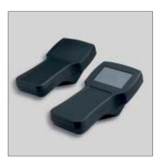
Beluga 220 - Ex consisting of: top part, bottom part, enclosure and board mounting screws, sealing rings, tongue-and-groove-System, with integrated seal. Open version comes complete with display screen and safety glass. Max. display board dimensions approx. 84 x 71.5 mm bzw. 86 x 70,5 mm
